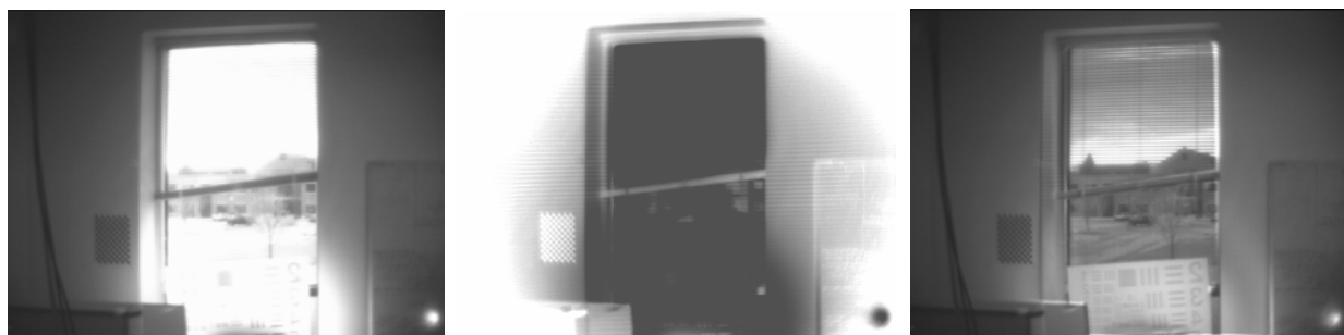
Figure 9: Sensor modulation for high dynamic range imaging. (a) Foam head scene. (b) Window scene. The first column shows the images captured with a white (full transmittance) pattern displayed on the SLM. The second column shows the feedback masks displayed on the SLM to attenuate the bright pixels present in the captured images. The third column shows the resulting images.
