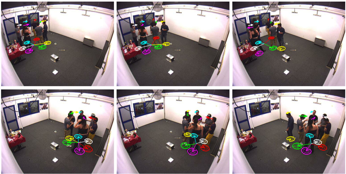
Fig. 12 Qualitative results on Cocktail Party dataset: estimated head pose ( arrows ), body pose (pie on the ground) and F-formations (connections on the ground)
