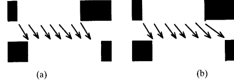
Fig. 1. Matching based on intensity is not sufficient to determine matching: (a) Point can be matched to any point with a similar intensity; (b) use of edges reduces the uncertainty in matching.
