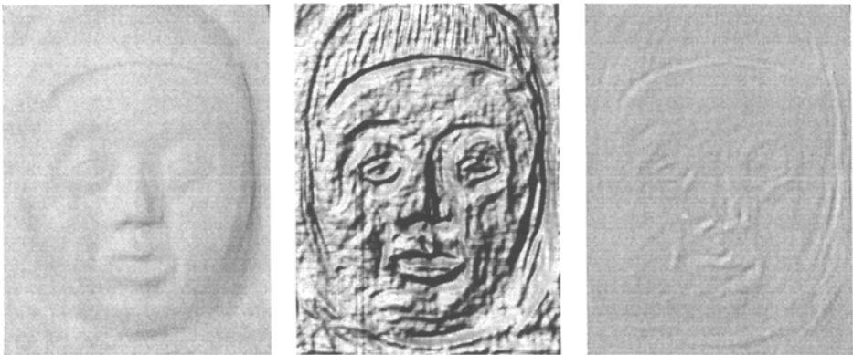
Fig. 5. Image of clay cherub figure, one of six feature maps, and shaded surface map, s(x, y) = g(f(x, y)) . Each feature is one coefficient of second degree polynomial fit to the local gray level surface.
